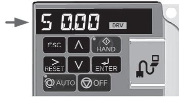
Press **↓** two times until the digital operator shows the parameter menu (PAR) then press **↵**.
