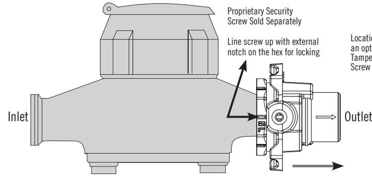
Ensure O-Ring is in Place Before Assembly
