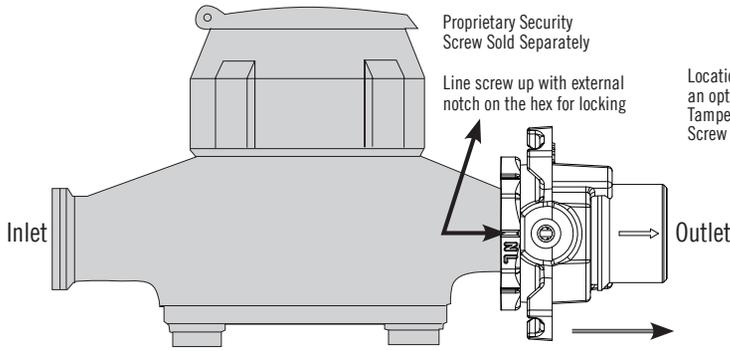
Ensure O-Ring is in Place Before Assembly
